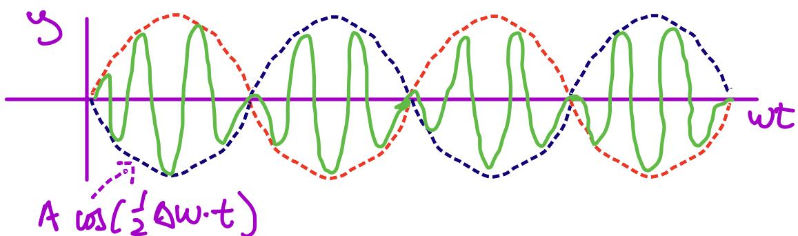
The signal  $\sin(\bar{\omega}t)$  is "modulated" by  $\frac{1}{2}\Delta\omega t \rightarrow$  "Beat freq" is  $|\Delta\omega|$
