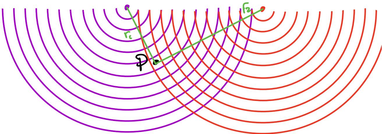
each wave has amplitude at point P given by
